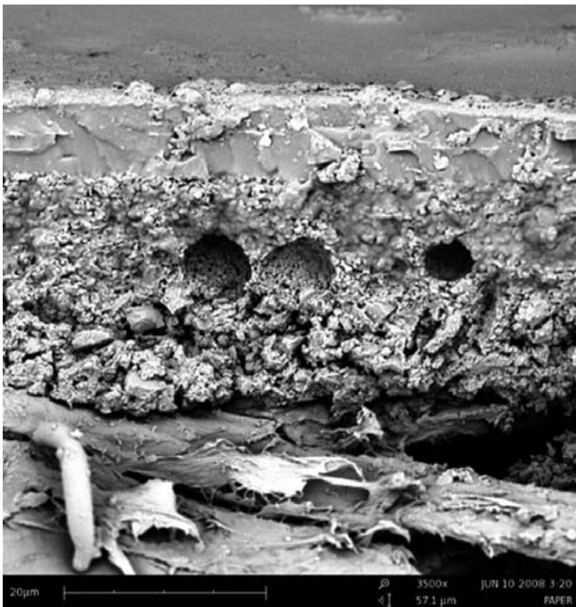
Image showing three distinct layers on coated paper. The bottom layer is the paper substrate, the middle layer (21.0 µm) a spray coating, and the top layer a final gloss finish (9.39µm). The large holes in the center are indicative of a faulty deposition in the coating process.
