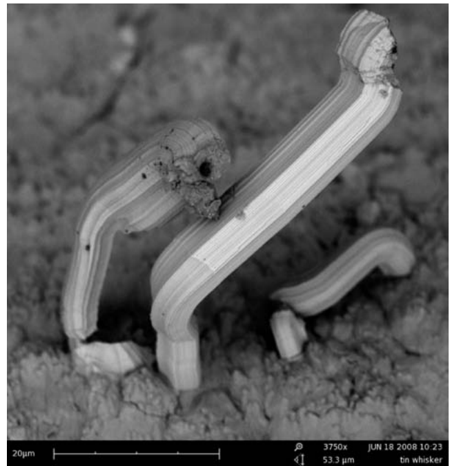
Tin whiskers at 3,750x magnification (Figure 4).
