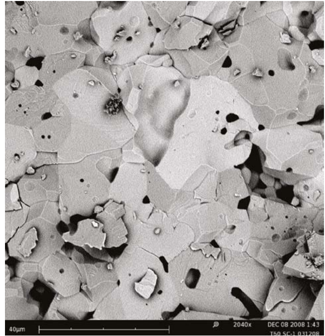
SEM picture of tabular alumina – there are almost no open pores present. The crystal size and boundaries can easily be seen here.
