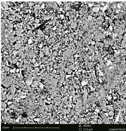
Coated-2 Magnified paper coating layer, individual coating particles; magnified 6,180x by Phenom.
