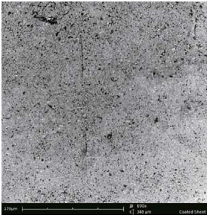
Coated-1 View of paper coating layer and overall coating structure; magnified 2,080x by Phenom.
