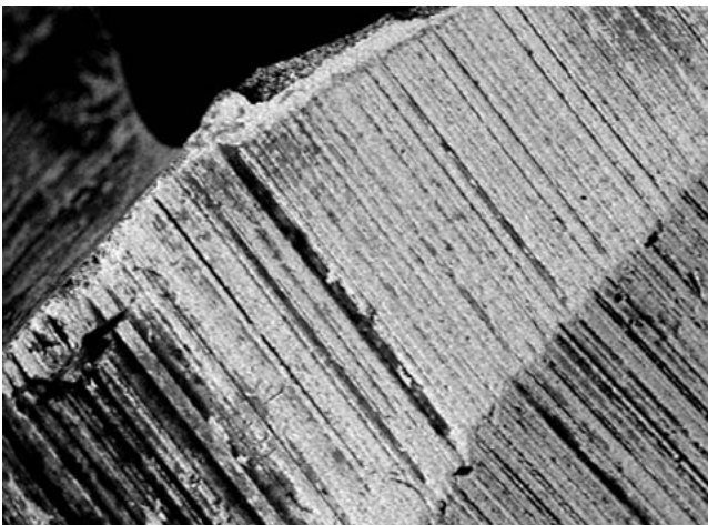
Drill bit, top view at 2900x magnification.
