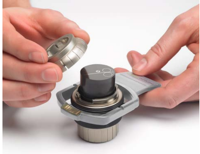
Inserting resin mount in metallurgical mount charge reduction sample holder.
