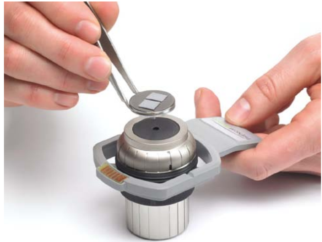
Inserting pin stub in charge reduction sample holder.
