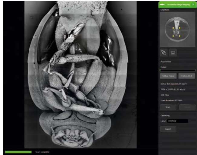
Example of large field of view automated image collection. The sample is a 3.15 x 4.15 mm ladybug that can be imaged completely at high resolution.
