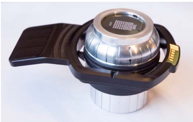
Special holder to support the polished metallurgical mounts up to 1 ¼ inch.
