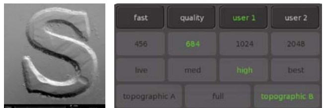
Image of the letter S (Euro coin) in topographical imaging mode (Figure 6).
