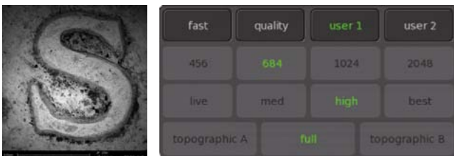
Image of the letter S (Euro coin) in compositional imaging mode (Figure 5).
